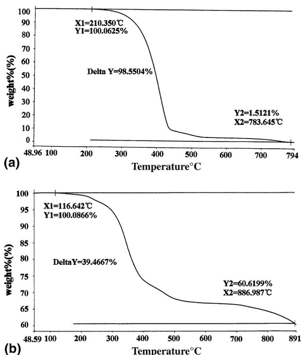
**Fig. 6** Thermogravimetric analysis of (a) fresh and (b) used grease sample
