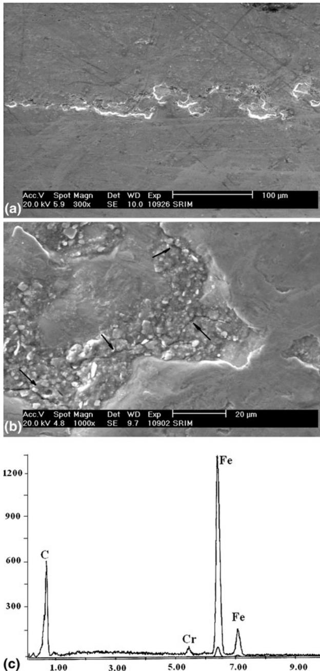
**Fig. 7** SEM and EDS of wear pits of outer perimeter of bearing inner ring. (a) Irregular pits, (b) magnified image of a single pit, and (c) EDS of pit
