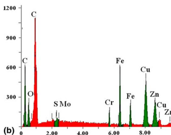
**Fig. 5** SEM and EDS of the used grease sample. (a) SEM micrograph and (b) EDS analysis
