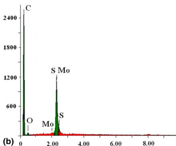
**Fig. 4** SEM and EDS of the fresh grease sample. (a) SEM micrograph and (b) EDS analysis
