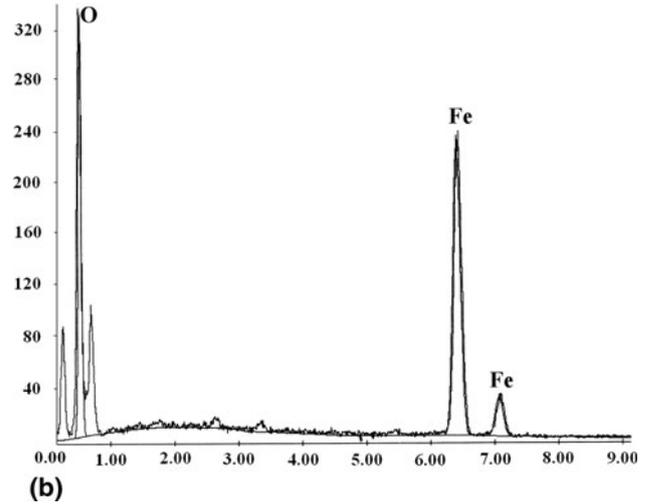
**Fig. 9** SEM and EDS of red-brown discolored zone on the outer perimeter of bearing inner ring (a) particulates and bands (b) EDS of particulates
