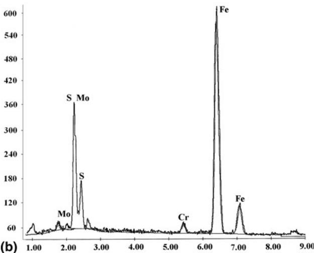
**Fig. 8** SEM and EDS of partial pits contained black particles. (a) Pits contained black particles and (b) EDS of black particles
