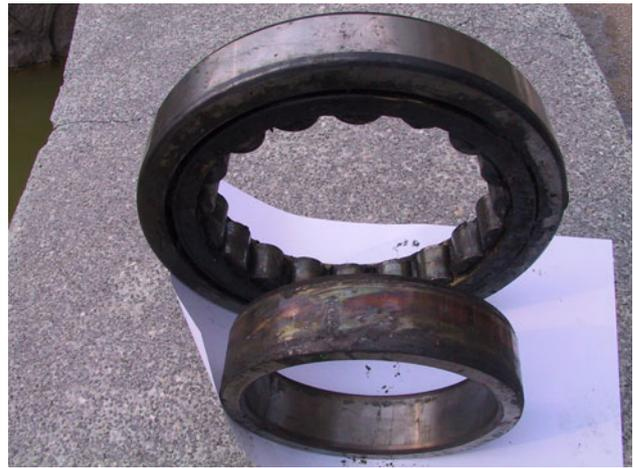
**Fig. 1** Dismounted samples of failure bearing
