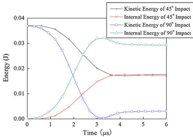
**Fig. 2** Internal and kinetic energies evolutions under normal and oblique impact
