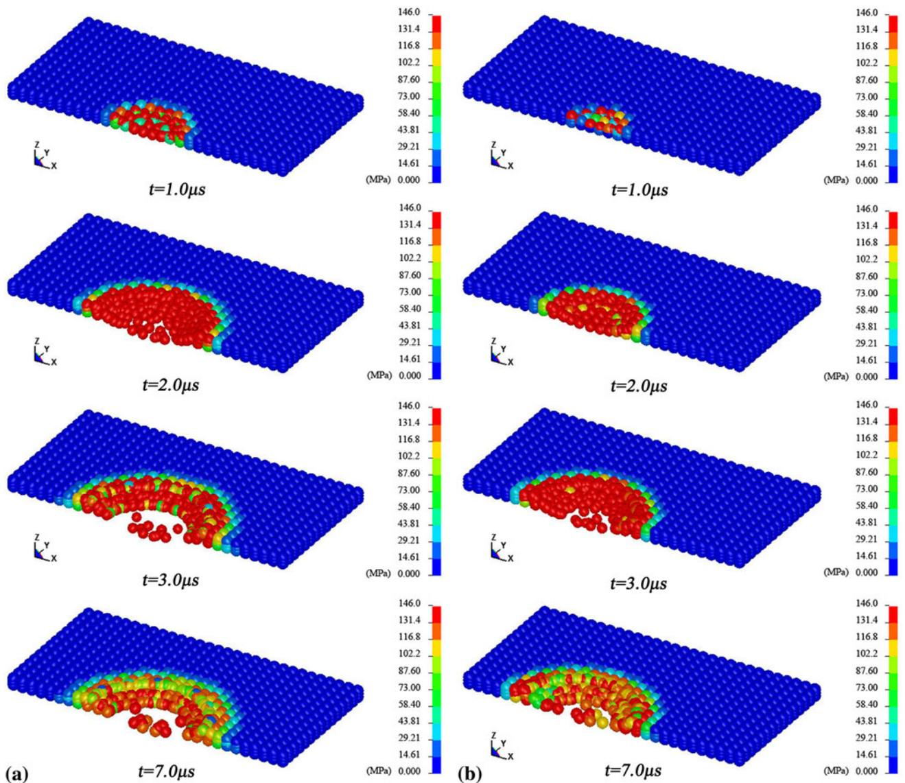
**Fig. 3** Stress distribution of the coating: (a) normal impact; (b) oblique impact
