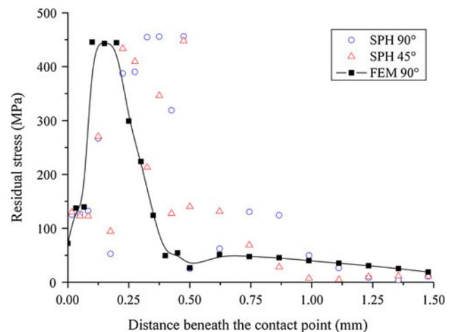
**Fig. 5** Residual stresses beneath the contact points (along the path of  $z$ -axis)
