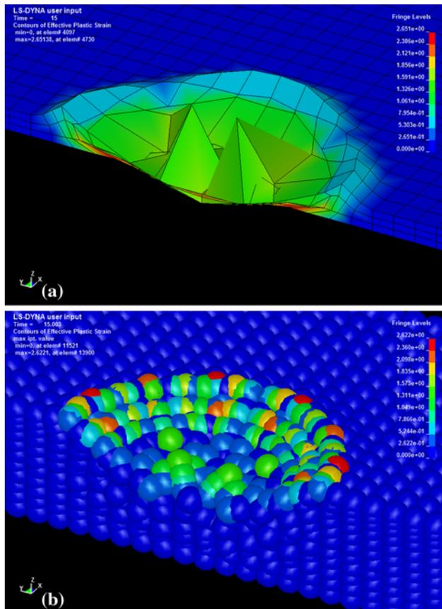
**Fig. 6** Plastic strain of the impacted area: (a) from FEM; (b) from coupled method (sole SPH method was same)
