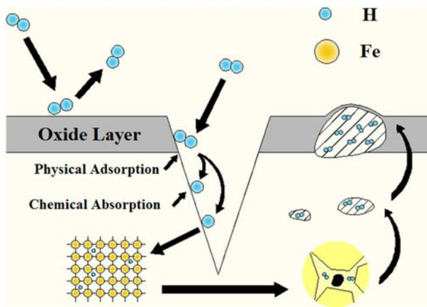
**Fig. 11** Main phenomena of hydrogen embrittlement according to Nelson [22]
