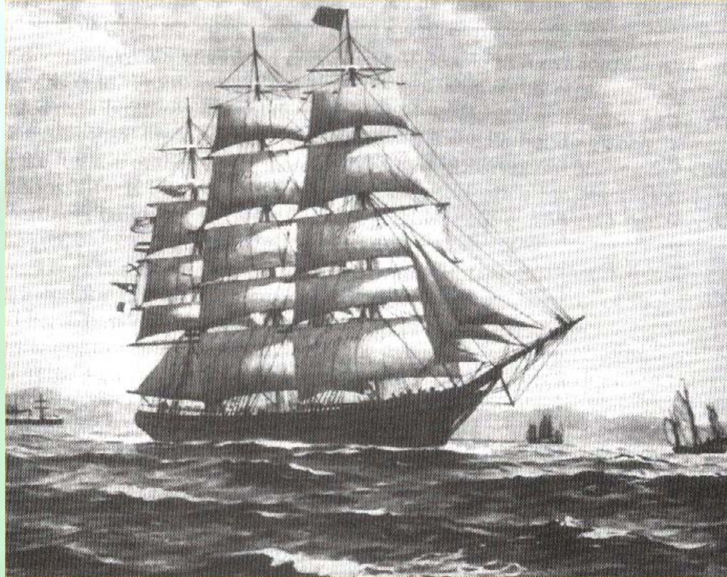
Figure 5.5 A fully rigged American sailing ship of the early 19 th century. Under good conditions this ship could extract thousands of horsepower from the wind. (Source: Corbis-Bettmann)
