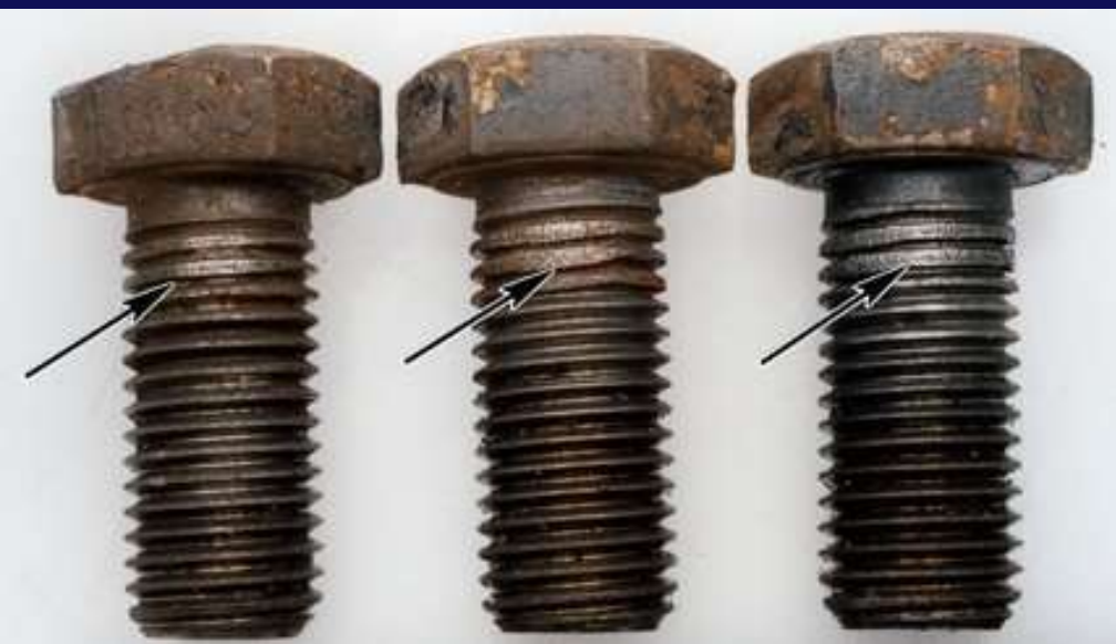
(a) 螺栓的微动磨损
