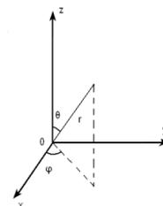
球坐标系是正交曲线坐标系,  $h_r = \sqrt{g_{11}} = 1$ ,  $h_\theta = \sqrt{g_{22}} = r$ ,  $h_\varphi = \sqrt{g_{33}} = r \sin \theta$ .
