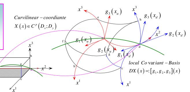
$$\gamma_{X}(t) \triangleq X \circ x(t) = X(x(t)) \in \mathbb{R}^{m} \Rightarrow \text{ind} \frac{d\gamma_{X}}{dt}(t) = D\gamma_{X}(t) = DX(x(t)) \cdot Dx(t) = \dot{x}^{i}(t)g_{i}(x(t))$$
