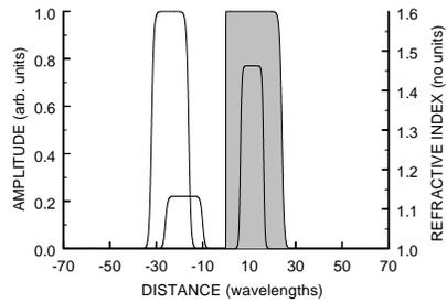
Fig. 4. Propagation of the vector potential from vacuum into a linear medium with a step-index for the entry and a gradient-index antireflection layer on the exit face. The shaded region is the profile of the index of refraction. The field travels to the right and the horizontal axis is scaled to the wavelength.
