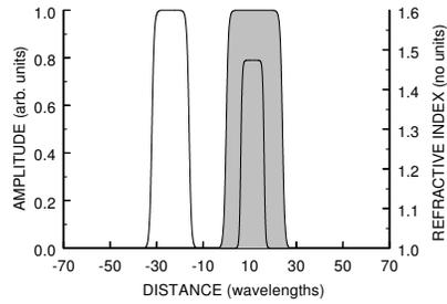
Fig. 1. Propagation of the vector potential from vacuum into a linear medium with a gradient-index antireflection layer on the the entry and exit faces. The shaded region is the profile of the index of refraction. The field travels to the right and the horizontal axis is scaled to the wavelength.
