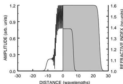
Fig. 3. Propagation of the vector potential from vacuum into a linear medium through a step increase in the refractive index. The shaded region is the profile of the index of refraction. The field travels to the right and the horizontal axis is scaled to the wavelength.
