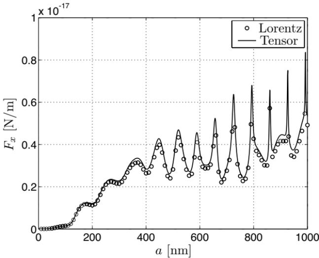
**Figure 6.** Radiation pressure on a magnetic cylinder ( $\mu_p = 3\mu_0$ ,  $\epsilon_p = \epsilon_0$ ) versus the radius  $a$ . The TE plane wave propagates in the  $\hat{x}$ -direction in free space ( $\mu_b = \mu_0$ ,  $\epsilon_b = \epsilon_0$ ), and the wavelength is 640 [nm]. The force is calculated by the divergence of the stress tensor (line) and the Lorentz force on bound currents and charges (markers).
