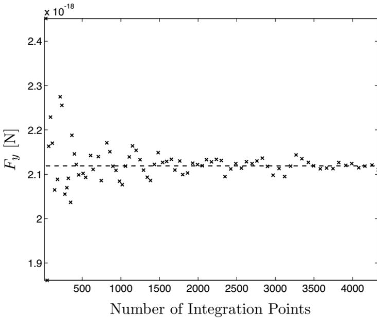
**Figure 3.**  $\hat{y}$ -directed force  $F_y$  versus the number of integration points for the direct application of the Lorentz force of (12). The configuration is the same as shown in Fig. 1. The dashed line is the force computed from the stress tensor of (9) with 100 numerical integration points on a concentric circle of radius  $R = 1.01a$ .
