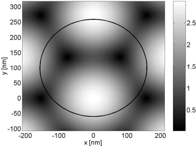
**Figure 1.** Incident electric field magnitude [V/m] due to three plane waves of free space wavelength  $\lambda_0 = 532$  nm propagating at angles  $\{\pi/2, 7\pi/6, 11\pi/6\}$  rad. The overlaid 2D particle is a cylinder ( $\epsilon_p = 2.56\epsilon_0$ ) of radius  $a = 0.3\lambda_0$  and infinite length in  $z$  with center position  $(x_0, y_0) = (0, 100)$  [nm]. The background medium is characterized by  $\epsilon_b = 1.69\epsilon_0$ .
