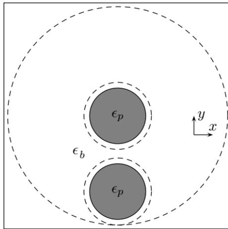
**Figure 4.** Two particles centered at  $(x, y) = (100, 0), (-300, 0)$  [nm] are subject to the incident field pattern of Fig. 1. The integration paths for the Maxwell stress tensor applied to the two particles are shown by the dotted lines. The sum of the forces on the two individual particles obtained by the smaller two integration circles is equal to the force obtained by integrating over the large circular integration path.
