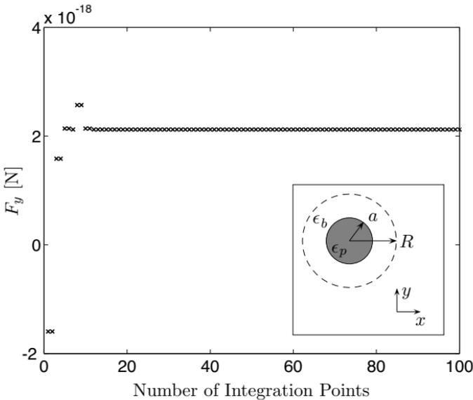
**Figure 2.**  $\hat{y}$ -directed force  $F_y$  versus the number of integration points used in the application of the Maxwell stress tensor in Eq. (9). The integration path, shown by the inset diagram, is a circle of radius of  $R = 1.01a$  concentric with the cylinder of radius  $a = 0.3\lambda_0$ . The configuration is the same as shown in Fig. 1.
