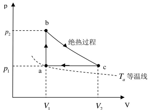
$$\Delta S_{\text{可逆}} = \Delta S_{ab} + \Delta S_{bc} + \Delta S_{ca} = nC_v \ln \frac{T_b}{T_a} + nC_p \ln \frac{T_a}{T_c} = nC_v \left( \ln \frac{T_b}{T_a} + \gamma \ln \frac{T_a}{T_c} \right)$$
