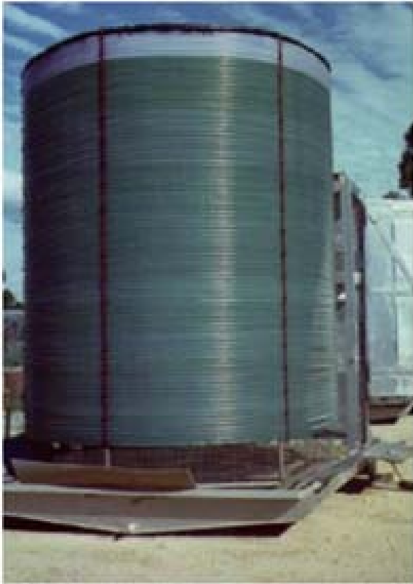
Fig. 4. A 1000 L helical tubular photobioreactor at Murdoch University, Australia. Courtesy of Professor Michael Borowitzka, Murdoch University.
