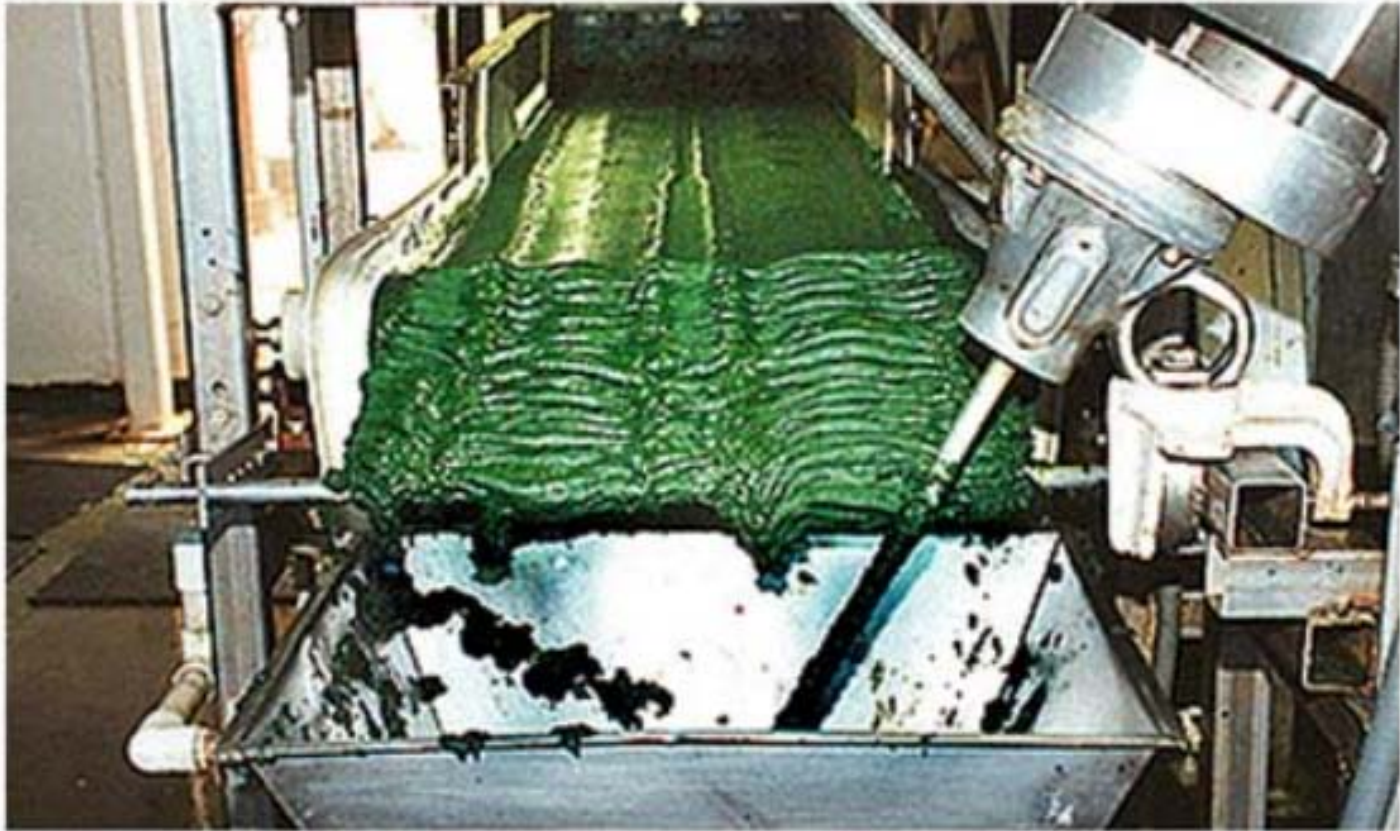
Fig. 5. Microalgal biomass recovered from the culture broth by filtration moves along a conveyor belt at Cyanotech Corporation ( www.cyanotech.com ), Hawaii, USA. Photograph by Terry Luke. Courtesy of Honolulu Star-Bulletin.
