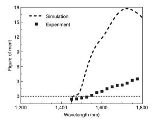
**Figure 5** | **Figure of merit for the 3D fishnet structure.** Plot of FOM against wavelength for the simulation (dashed line) and experiment (squares). The lower experimental FOM is due to reduced transmission resulting from fabrication imperfections. The experimental FOM reaches 3.5 at 1,775 nm, where Re(n) = -1.23.
