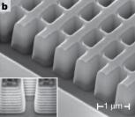
Figure 1 Diagram and SEM image of fabricated fishnet structure.
